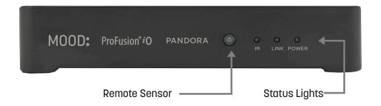
The ProFusion *i*O Pandora front panel has three status indicator lights and a sensor for infrared remote control. The remote sensor must not be blocked if use of the remote control is desired.
