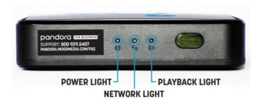
The ProFusion *i*H Pandora front panel has three status indicator lights and a sensor for infrared remote control. The remote sensor must not be blocked if use of the remote control is desired.
